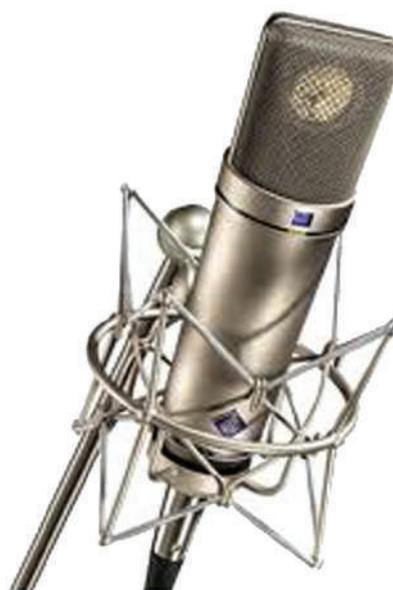
**Fig. 18.10 (b)** Condenser microphone
