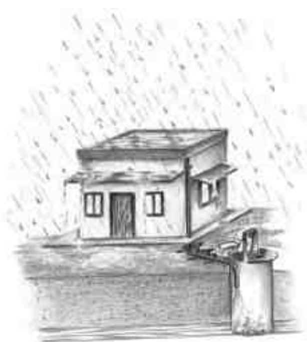
(b) Recharge through Abandoned Dugwell
