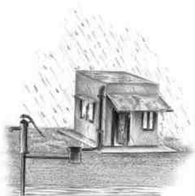
(a) Recharge through Hand Pump
