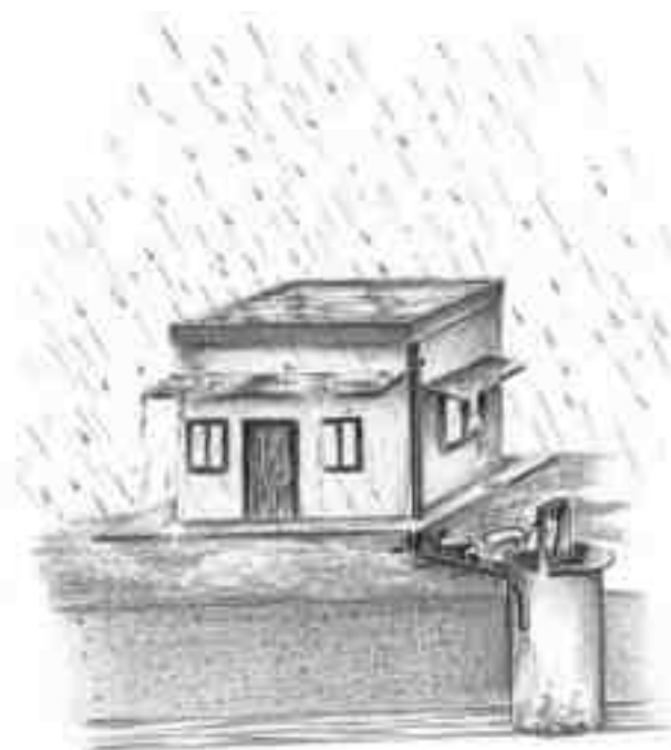
(b) Recharge through Abandoned Dugwell
