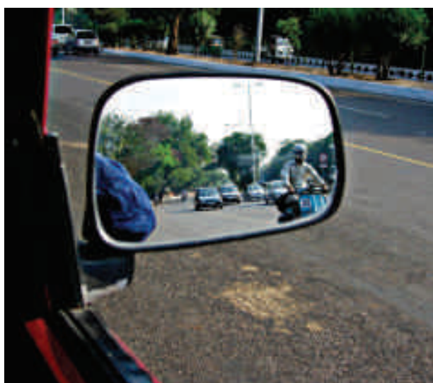
Fig. 15.20 Convex mirror as side view mirror
