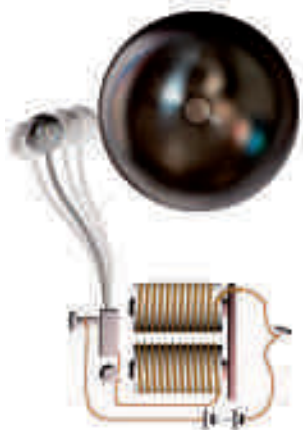
Fig. 14. 20 Circuit of an electric bell
