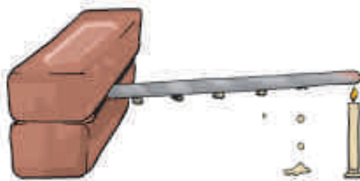
Fig. 4.7 Flow of heat through a metal strip
