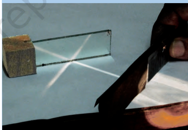
Fig. 16.1 : Arrangement for showing reflection
